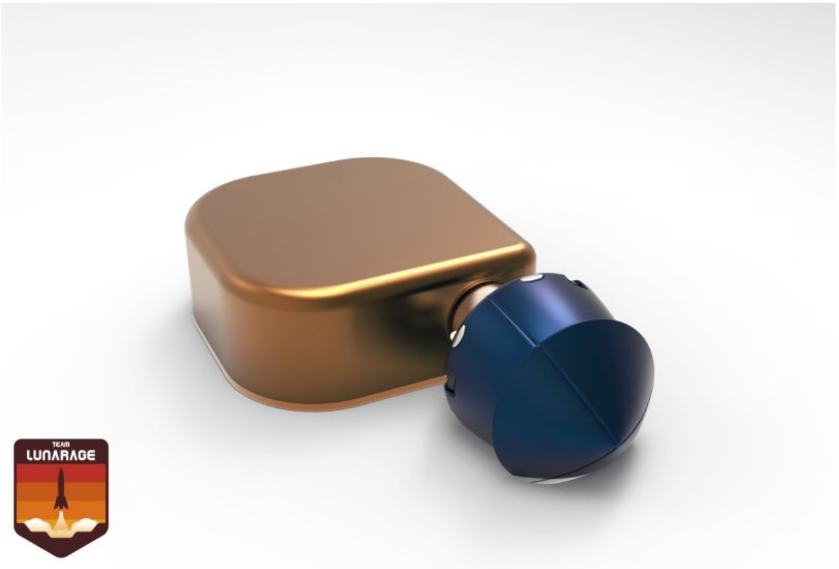
Figure 15. Render of excavation winch module.
