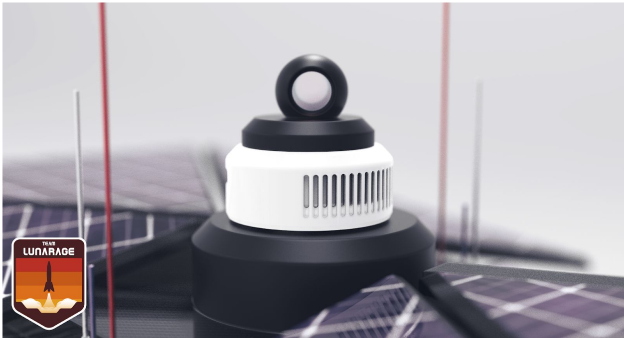
Figure 23. Render of central LiDAR and vision tracking system.
