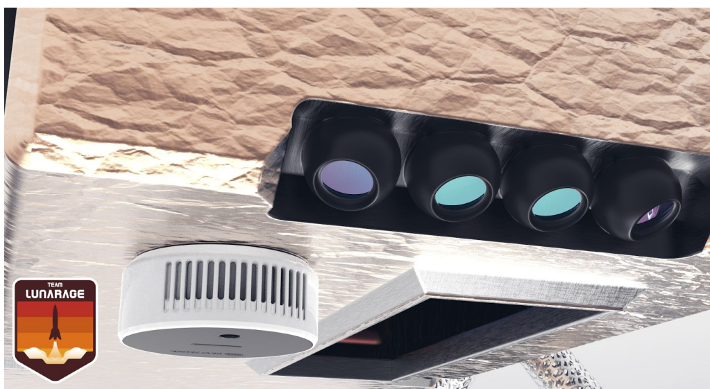
Figure 21. Render of LiDAR and vision system.
